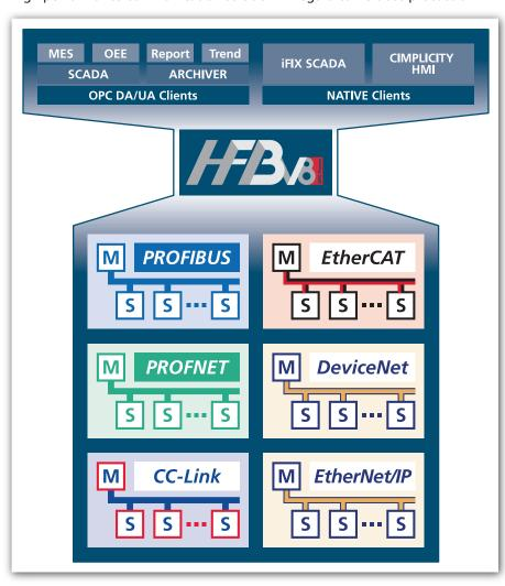
The specialized solution for the fieldbus protocols PROFIBUS, PROFINET, EtherCAT, EtherNet/IP, DeviceNet and CC-Link with Hilscher CIF/CIFX cards and NetHOST gateways.
