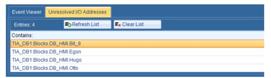
This new window shows all iFIX I/O addresses and OPC Item Ids which could not be resolved by the background server. An unresolved I/O address means that
