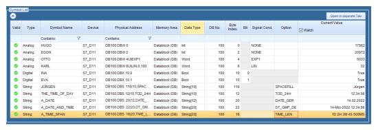
The driver now allows to define symbols for I/O addresses of communication ways with physical addressing (e.g. S7 300/400/1500 TCP Absolute).
