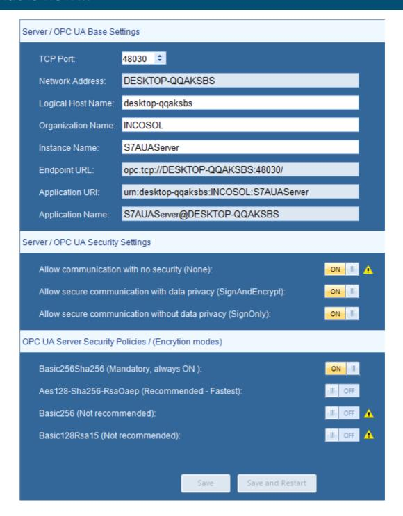
The configuration of the OPC UA Server and the entire certificate management (even the request from a GDS) is integrated in the S7A Power Tool.
