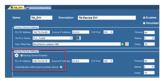
When a backup device IP address is configured and the **Backup Device Enabled** check box is checked, the driver automatically switches the IP connection to this backup address in case that the primary connection becomes disturbed.
