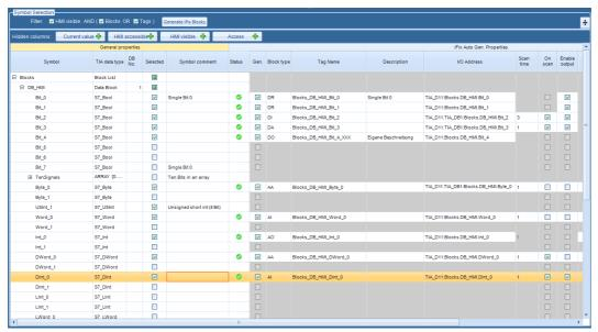
The symbol selection tree in the Power Tool's TIA data block configuration dialog has been extended by addition columns which allows to directly configure and generate iFIX database blocks from within the Power Tool. The following data block fields can be configured by this way:
