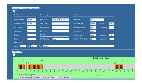
The Power Tool now provides a tool which allows the monitoring of the client access to the data byte of a single driver data block.
