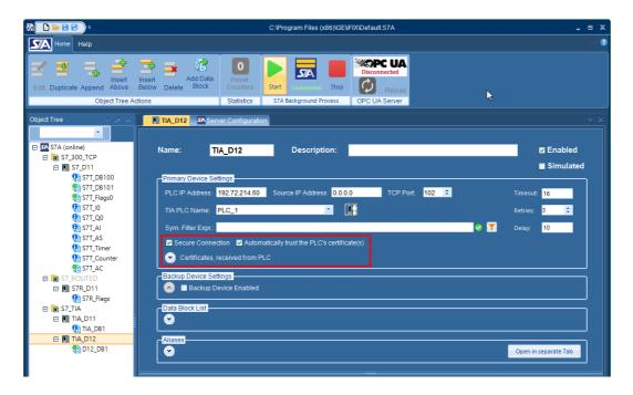
In the expandable panel 'Certificates received from PLC', you can view detailed information about the certificates received by the PLC.
