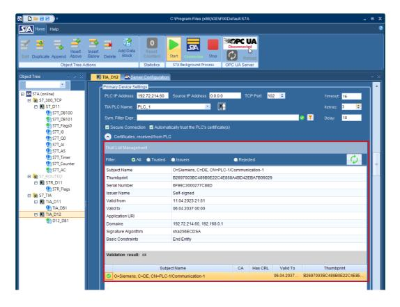
Please note that secure communication must be explicitly activated on the PLC side. The TIA Portal offers the 'Security Wizard' in the 'Protection & Security' settings for the PLC CPU for this purpose:
