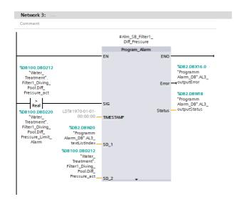
This new S7A function also enables the alarm texts defined in the TIA project (from PLC alarm text lists), which are also transmitted via an alarm associated value (parameters SD\_1 to SD\_10), to be made available to the S7A clients. Combined with the INCOSOL DAX block (extended digital alarm block for iFIX) the PLC message texts can then be sent directly as alarm texts to the iFIX alarm system.
