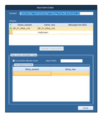
In this dialog you can enter an alias name individually or have it generated automatically. With automatic generation you can, for example, remove irrelevant symbol path elements (e.g. the group name 'Blocks') or replace long symbol path elements with shorter ones. In addition, you can define a prefix to be placed in front of the alias name.
