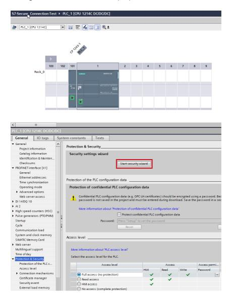
The S7A driver can only establish a secure connection once the PLC has been downloaded with the certificate required for encryption via the TIA Portal.
