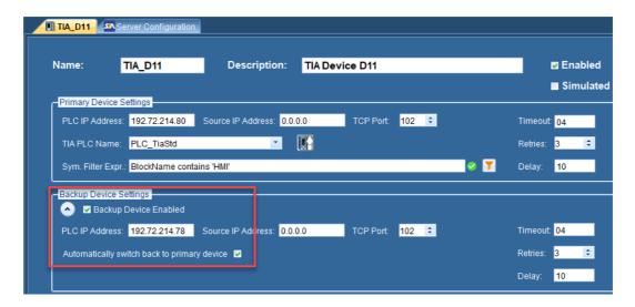
When a backup device IP address is configured and the **Backup Device Enabled** check box is checked, the driver automatically switches the IP connection to this backup address in case that the primary connection becomes disturbed.
