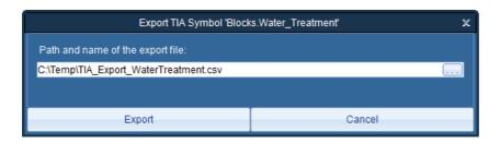
In this version, the structure (the number and sequence of the exported fields) is fixed. In a later S7A version, the fields and their sequence will be freely selectable.
