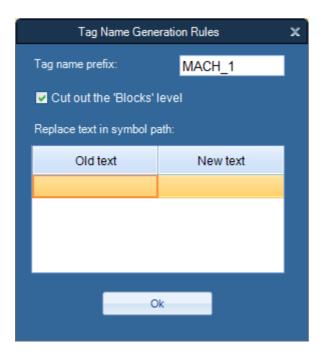
The automatic iFIX tag name generation can be controlled by various options.
