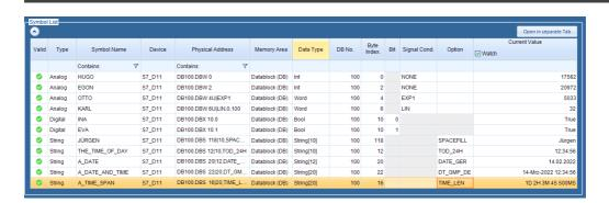
The driver now allows to define symbols for I/O addresses of communication ways with physical addressing (e.g. S7 300/400/1500 TCP Absolute). These symbols can be used as iFIX I/O addresses or OPC Item Ids as an alternative to the physical I/O address. Means, a symbolic name and I/O address are interchangeable.
