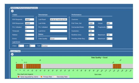
The Power Tool now provides a tool which allows the monitoring of the client access to the data byte of a single driver data block.
